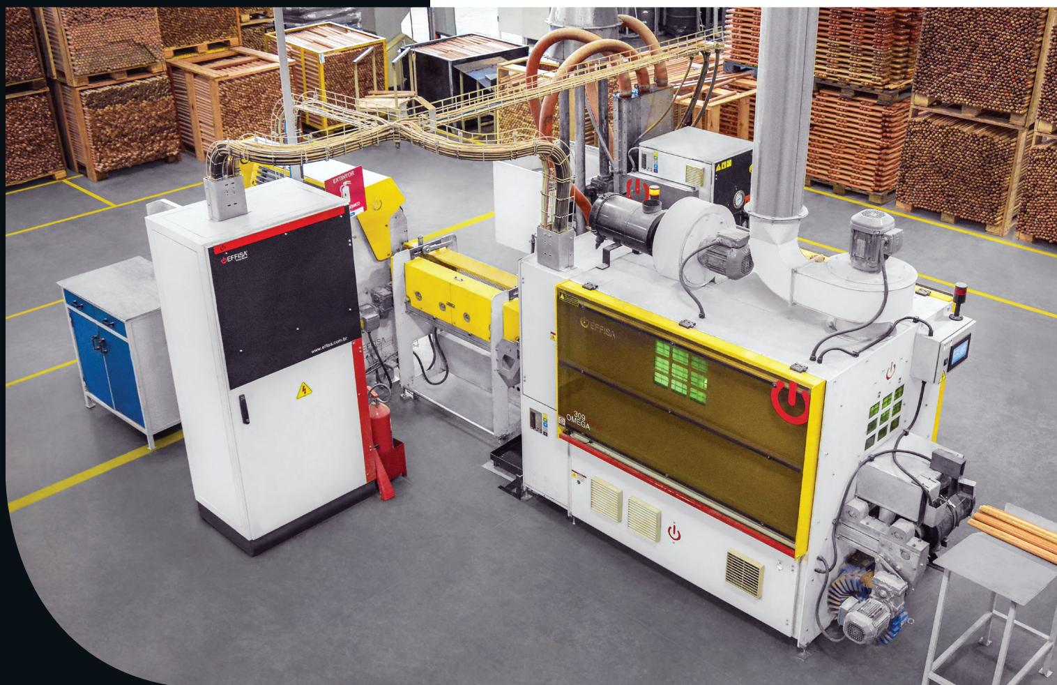
Tramontina Multi now features an automated system to varnish wooden handles in its tools lines. The products gain a high-quality finish and, consequently, do even more beautifully well at points of sale. In addition to increased productivity, the automation of this process reduces manufacturing costs since the varnish can be reused, which also avoids residue and fumes in the work environment.
